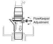
The parts used to connect the hose, and the sequence in which they are installed depends on the type of skimmer.
