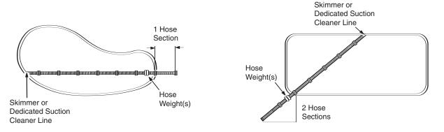
Position the hose weight(s), two for US/Mexico installations and one for Canadian, in the middle of the second hose section, about 60" (1.5 m) back from the end of the hose.
