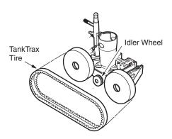
8. Use a ruler to measure the distance from the ground line to the inside lip of the upper track. Slide the rear double-side wheel back until proper tension is achieved at 6-3/4". Tighten axle block screws.
