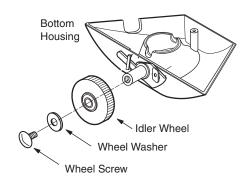
4. Loosen and remove both the front and back double-wheel side wheel screws, wheel washers and wheels. Remove and store or discard both double-wheel side axles. Install the new axle blocks leaving the back wheel axle screws loose for further adjustment.
