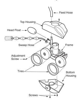
Push the axle tee screw through the large hole in the new bottom housing. Mount the swing axle using swing axle tee. Install tap screw to secure swing axle.
