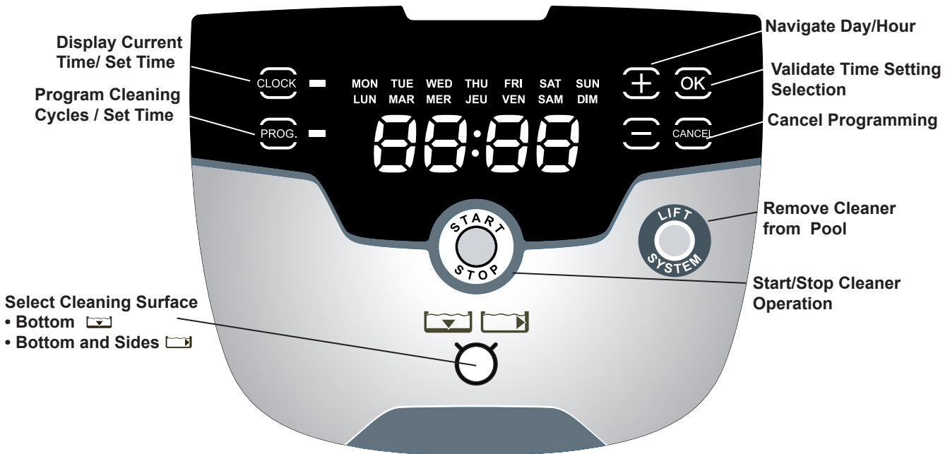
Figure 16. 9400 4WD / P94 4WD Control Unit Functions
