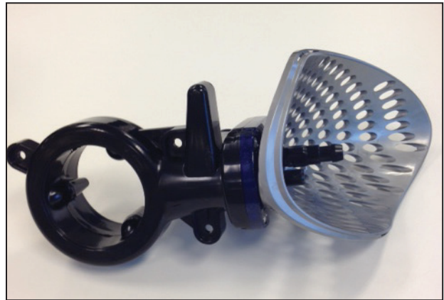
Figure 7. Water management system and rear housing removed
