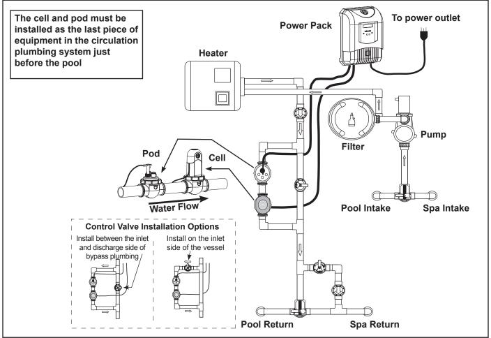
Figure 19. Example of Bypass Installation
