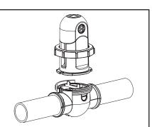
Figure 25. Remove the Cell
