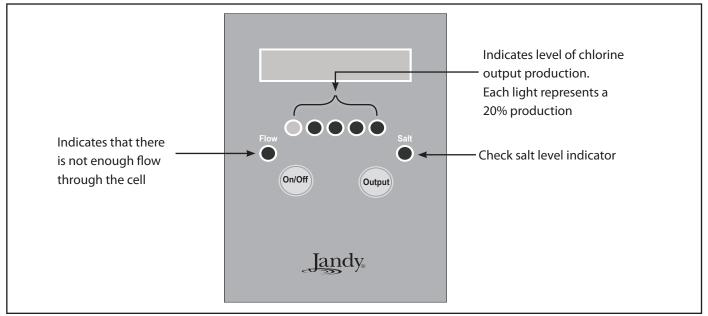
Figure 23. **Control Panel on the Power Pack**
