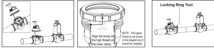
Figure 13. Installing Pod and Cell Figure 14. Locking Ring Alignment Figure 15. Locking Ring Tool
