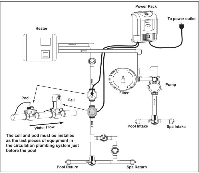
Figure 1. Example of Installation
