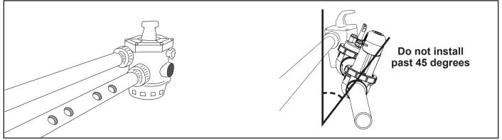
Figure 20. Example of Alternative Installation
