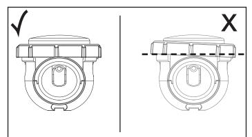
Figure 28. Locking Ring Level
