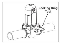
Figure 24. Undo Locking Ring
