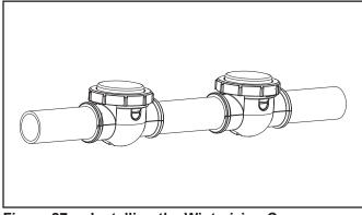
Figure 27. Installing the Winterizing Cap
