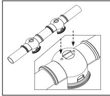
Figure 7. Marking Pipe for Drilling Feeder Holes
