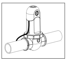
Figure 17. Attaching Terminal Cap
