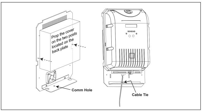
Figure 19. Accessing and Wiring to the Power PCB
