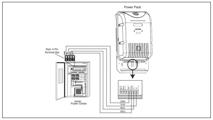
Figure 21. Communication Wiring between Power Pack and AquaLink RS Control System or PDA Network
