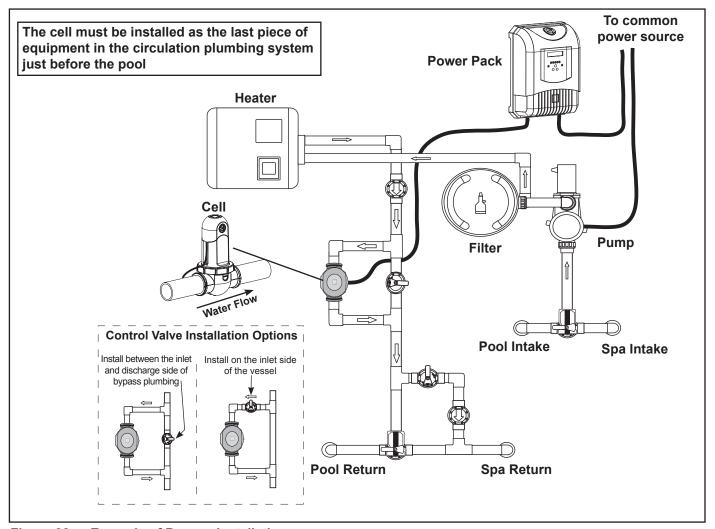
Figure 22. Example of Bypass Installation
