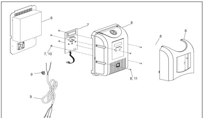
Figure 31. Power Pack Exploded View
