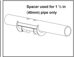
Figure 9. Pipe Spacer
