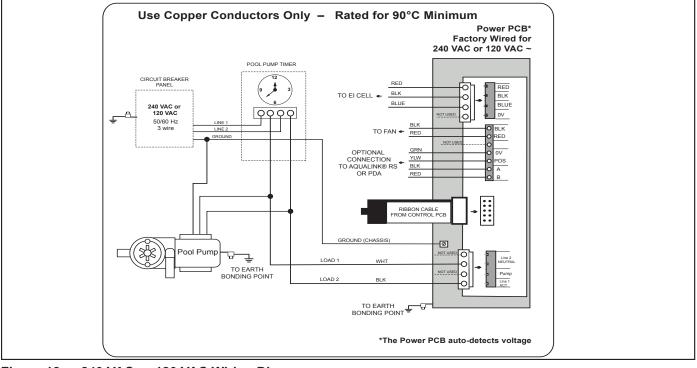
Figure 18. 240 VAC or 120 VAC Wiring Diagram
