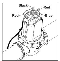
Figure 16. Connecting Cell Leads Figure 17.
