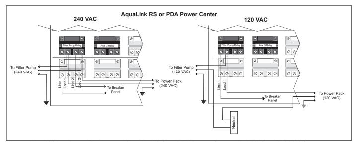
Figure 20. Wiring Power Pack to an AquaLink RS or PDA Power Center (240 VAC and 120 VAC)
