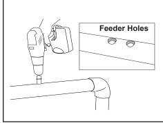
Figure 8. Drilling Feeder Holes
