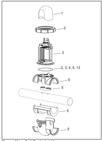
Figure 30. Winterizing Cap and Locking Ring Tool
