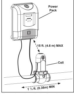
Figure 3. Installation Requirements
