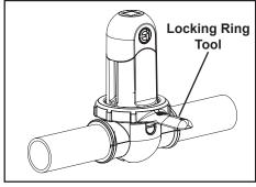
Figure 25. Undo Locking Ring
