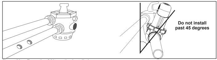
Figure 23. Example of Alternative Installation
