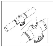
Figure 7. Marking Pipe for Drilling Feeder Holes
