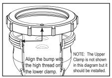
Figure 13. Locking Ring Alignment
