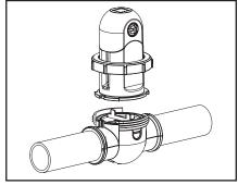
Figure 26. Remove the Cell
