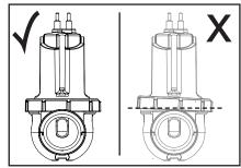
Figure 15. Locking Ring Level
