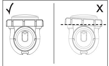
Figure 29. Locking Ring Level
