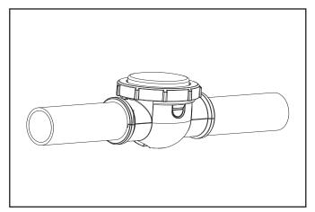
Figure 28. Winterizing Cap Installed
