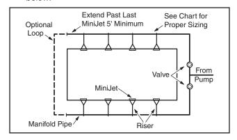
When the MiniJets are lined up to project water streams of equal distance, cut the riser to equal lengths. When the MiniJets are not set in lines parallel to the pool ledge, valve each MiniJet separately.
