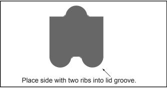
Figure 3. **Cross Section of Lid Seal**
