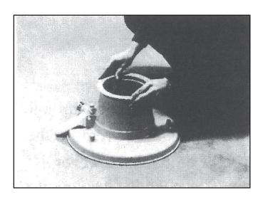
**1.** Press bag ring into body as shown until snap is heard. Use firm hand pressure; do not pound.
