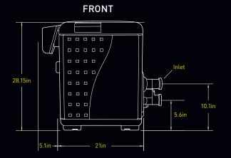
NOTE: Dimensions are identical on all JXi heater models
