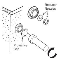
5. At startup, select and insert the applicable restrictor nozzle if required for the installation.
