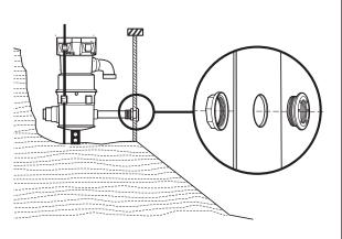
Figure 6. Deck Canister Installation (Vinyl Liner Pools)
