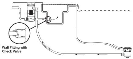
Figure 3. Orientation of the Internal Check Valve
