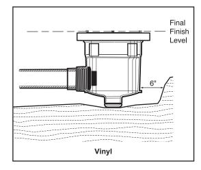
Figure 7. Floor Canister Installation
