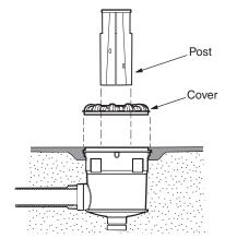
Figure 11. Floor Canister Post and Cover
