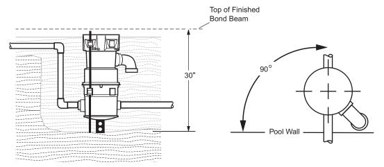
Figure 4. Deck Canister Installation
