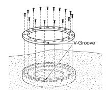
Figure 9. Installing the Locking Ring, Post, and Cover
