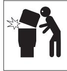
Follow all filter manufacturer's instructions. Never attempt to assemble, disassemble or adjust the filter when there is pressurized air in the system. Starting the pump while there is any pressurized air in the system can cause the filter lid to be blown off, which can cause death, serious personal injury or property damage.
