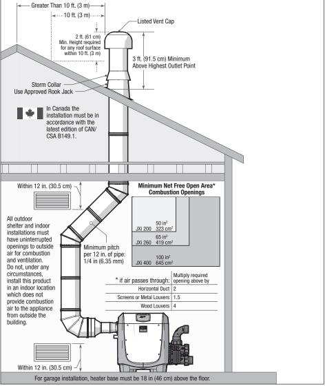
Figure 4. Indoor and Outdoor Shelter Installation
