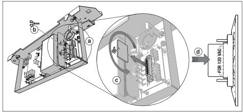
Figure 18. Input Conversion Process
