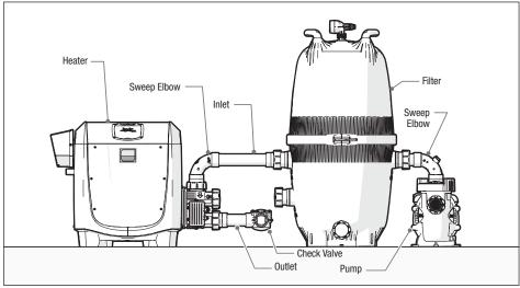
Figure 11. Versa Plumb Heater Inlet
