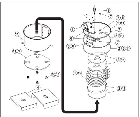
Figure 44. ASME Combustion Chamber Components
