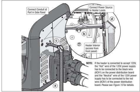
Figure 17. Main Wiring Connections
