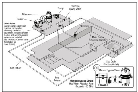
Figure 9. Typical Water Piping Configuration
