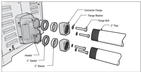
Figure 38. 2" Threaded Inlet Pipe
