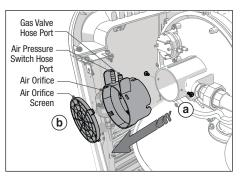
**TIP:** When removing the air hoses form the air orifice, mark the hoses with tape or a marker to help with reassembly.
