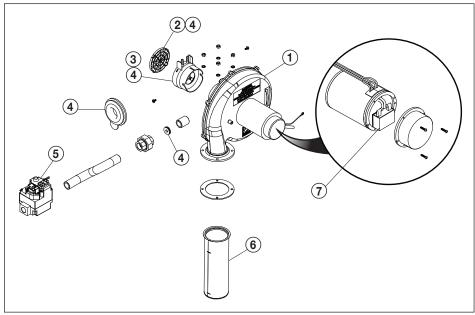
Figure 31. Burner Components
