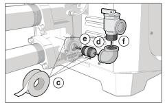
Figure 41. Install the Elbow
