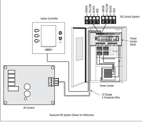
Figure 19. Wiring the JXi to a Zodiac® Remote
