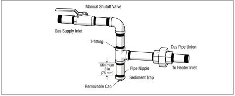
Figure 8. Manual Shut-off Valve and Sediment Trap
