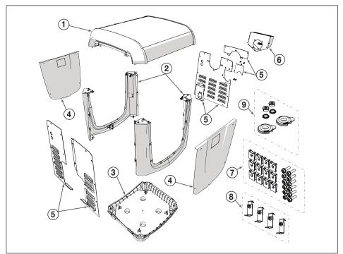
Figure 43. ASME Cabinet Assembly Components
