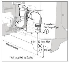
Figure 42. Install the Discharge Pipe
