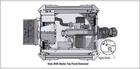
Figure 26. Remove Heater Top to View Sight Glass
