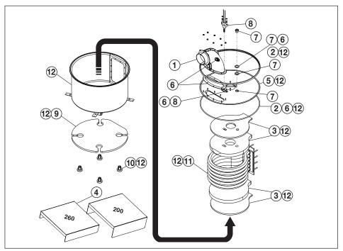
Figure 30. Combustion Chamber Components
