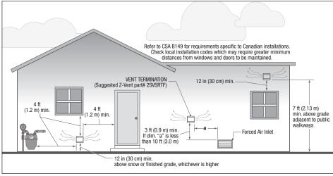
Figure 7. Side Wall Vent Termination
