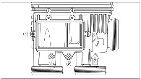
Figure 27. Header Bypass Reassembly Torque Pattern
