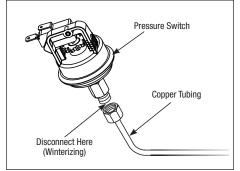
Figure 25. Water Pressure Switch Copper Tubing (Siphon Tube)
