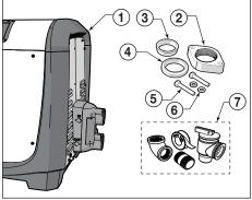
Figure 36. Pressure Relief Valve Components
