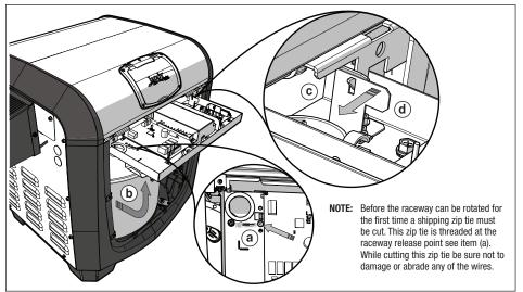
Figure 16. Raceway Rotation for Service Access
