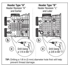
Figure 14. Identifying Header Design
