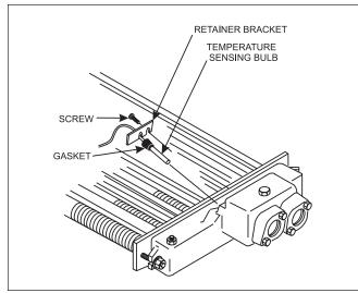
Figure 10. Temperature sensing bulb
