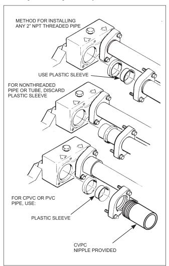
Figure 13. Piping installation
