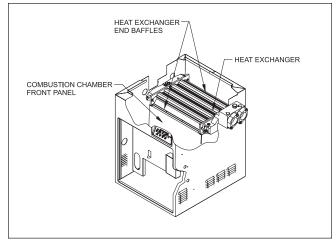
Figure 12. Heat exchanger and end baffles
