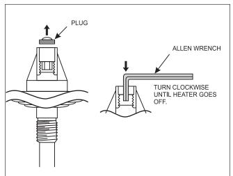
Figure 21. Pressure Switch Adjustment
