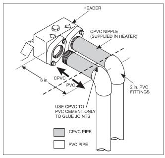
Figure 14. Plastic piping connections
