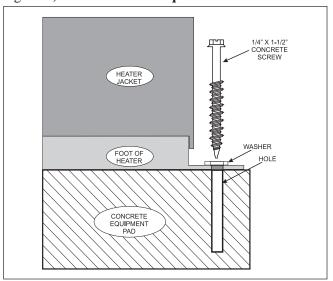
Figure 4. Anchor Heater to Equipment Pad.
