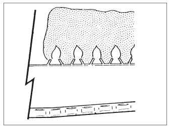
Figure 24. Main Burner Flame
