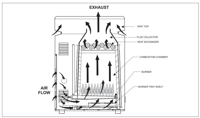
Figure 26. Atmospheric Combustion System
