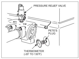
Figure 15. Thermometer and pressure relief valve
