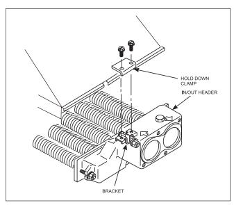
Figure 9. Flue collector hold-down brackets
