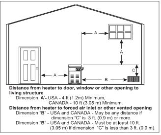
Figure 3. Outdoor Heater Installation
