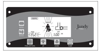
Figure 25. Typical Service Code Display
