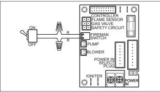
Figure 19. ON/OFF Type remote switch
