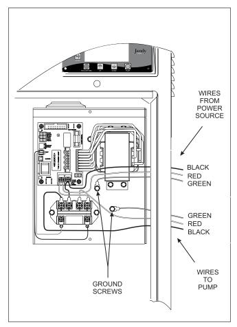
Figure 17. Field Wiring Connections (230V Shown)
