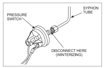
Figure 23. Pressure switch copper tubing
