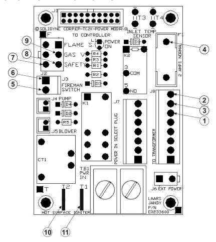
Figure 27. Power and Control Circuit Test Points
