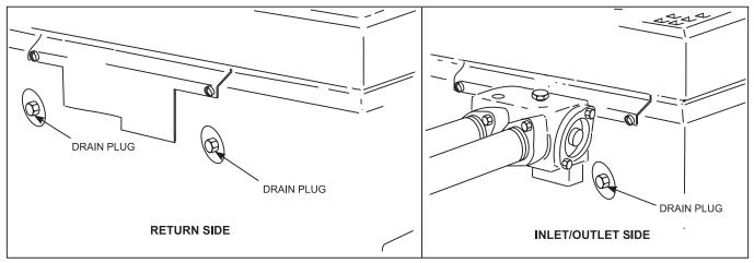
Figure 22. Heater drain locations
