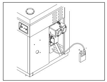
Figure 40. Collector pressure measurement.
