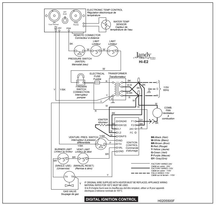
Figure 15. Wiring diagram, Hi-E2 pool heater.
