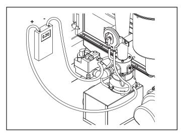
Figure 35. Gas pressure offset measurement.
