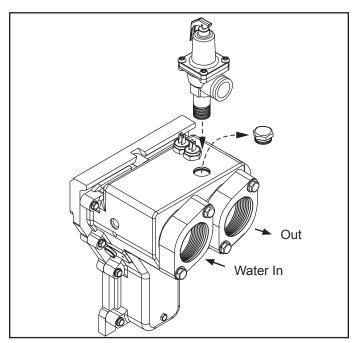
Figure 22. Pressure relief valve installation.
