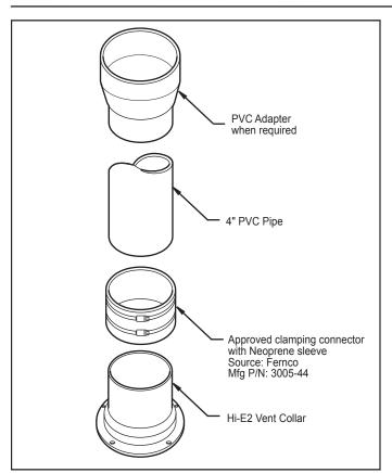
Indoor vent connection, Hi-E2 pool heater. Figure 7.
