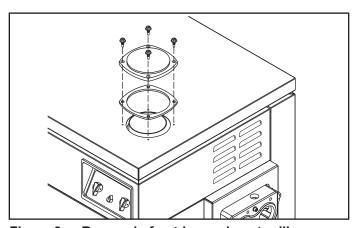
Figure 3. Removal of outdoor exhaust grille.
