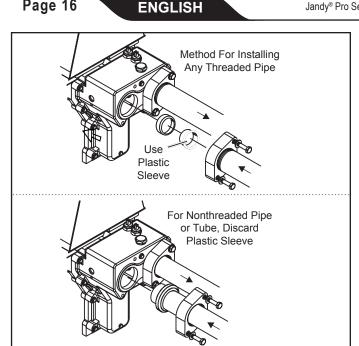
Figure 21. Piping to heater.
