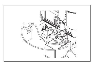
Figure 37. Unfired venturi differential measurement.
