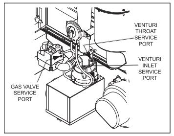
Figure 33. Venturi flow system components.
