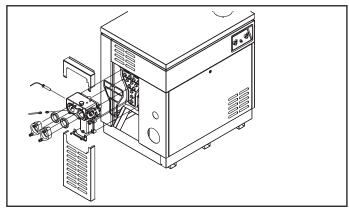
Figure 19. Water connection reversal.
