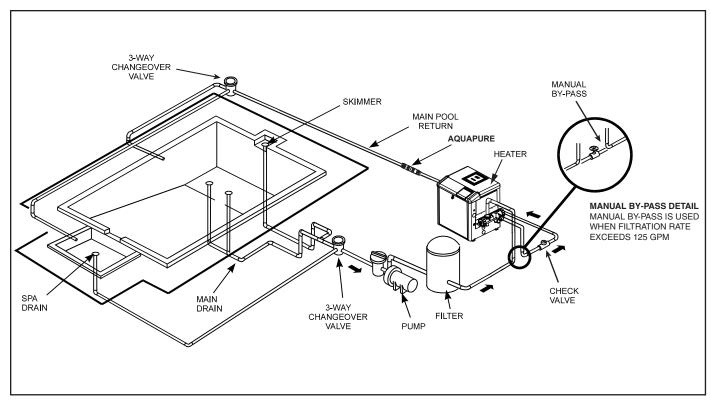
Figure 20. Typical water piping.
