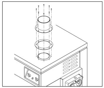
Figure 4. Vent collar assembly for indoor installation.
