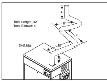
Figure 6. "One-pipe" installation.
