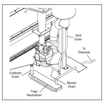
Figure 11. Condensate drainage components.
