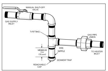
Figure 13. Manual Shut-off Valve and Sediment Trap.
