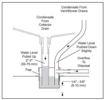
Figure 12. Condensate drain and trap.
