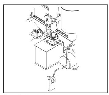
Figure 39. Venturi inlet pressure measurement.
