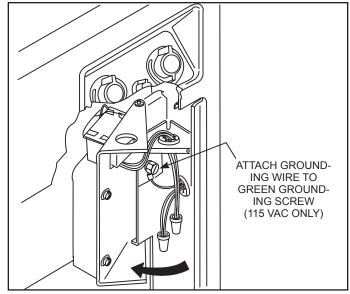
Figure 14. Field wiring connections.
