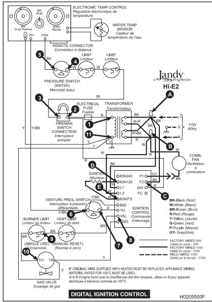
Figure 32. Wiring diagram with test points.
