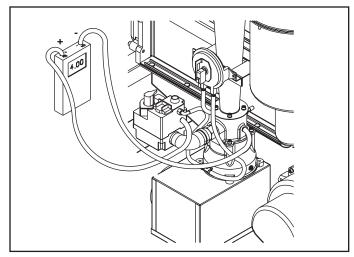
Figure 34. Gas orifice differential measurement.
