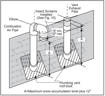
Figure 9. Vent and combustion air terminals at roof. located at a public walkway.
