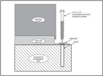
Figure 2. Anchor heater to equipment pad.
