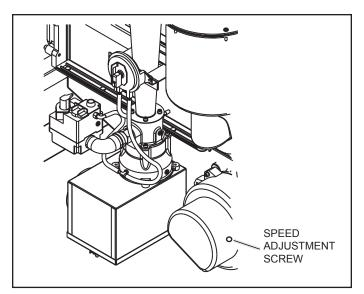
Figure 38. Blower Speed Adjustment.
