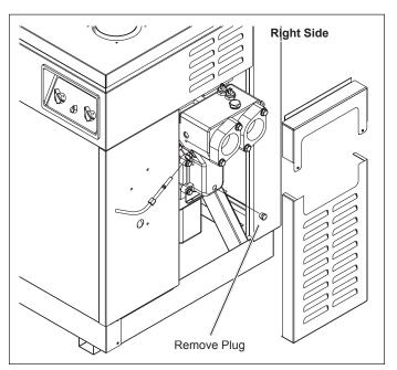
Figure 28. Water header draining.
