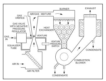
Figure 30. Combustion system diagram.
