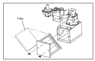
Figure 31. Air filter replacement.
