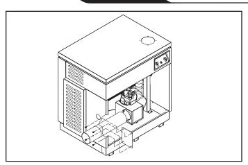
Figure 5. Connection of combustion air pipe to heater.
