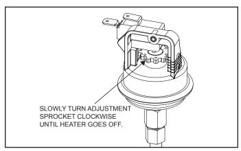
Figure 24. Adjustment of pressure switch.
