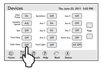
NOTE If a solar sensor is not installed, EXTRA AUX replaces SOLAR HEAT and may be used to control an auxiliary piece of equipment (see the following Section 9.7, "Auxiliary Equipment" to turn on or off EXTRA AUX).
