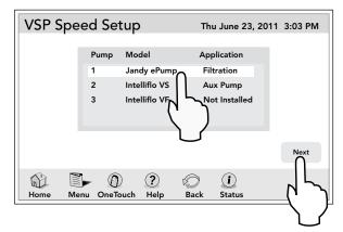
Select the pump/model and click the NEXT button to display the eight (8) speed VSP SETUP screen.
