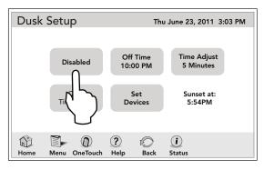
On the DUSK SETUP screen, click the OFF TIME button and enter the desired time
