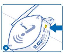
Within 2 minutes, the yellow LED should stop blinking. When the green LED illuminates, the iAguaLink is now connected.
