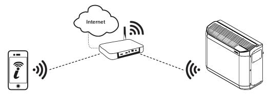
The Z400iQ heat pump may be controlled by remote, from a smartphone or tablet, via the iAquaLink™ app available for iOS and Android systems.
