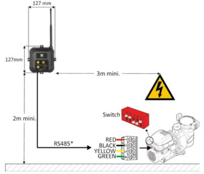
\*DO NOT connect the device to any source of mains or high voltage; the device operates on RS485 power levels ONLY.
