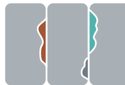
GALVANIC CORROSION OCCURS WHEN DIFFERENT METALS TOUCH
