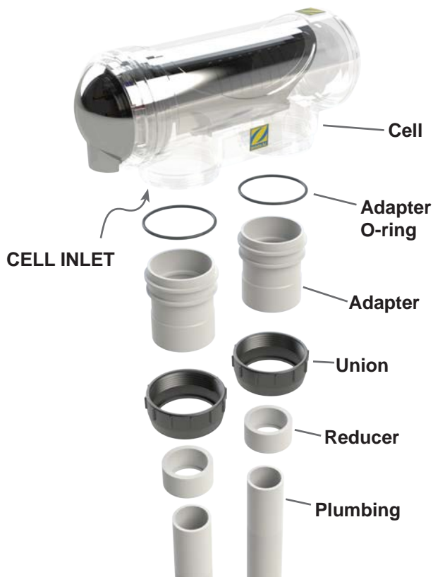
Figure 5. Cell Plumbing Assembly
